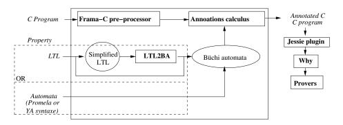
Figure 5.2: Plug-in Structure
