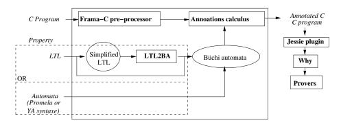
Figure 5.2: Plug-in Structure
