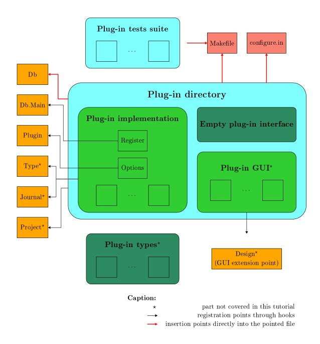
Figure 2.2: Kernel-integrated Plug-in Integration Overview.
