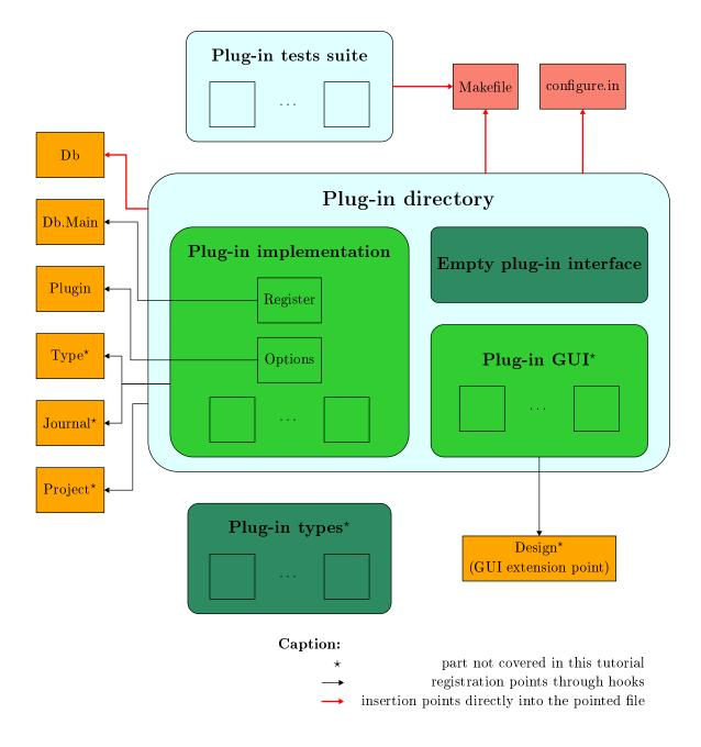
Figure 2.2: Kernel-integrated Plug-in Integration Overview.
